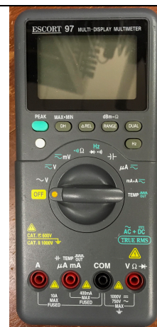
Figure 6 CAT III Multimeter, mostly used for current measurement
