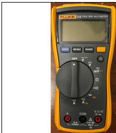
Figure 5 CAT III Multimeter, mostly used for voltage measurement
